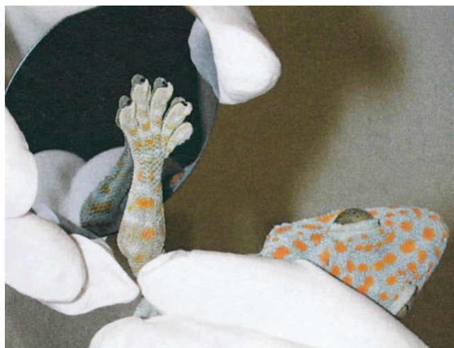
Fig. 2. Tokay gecko ( Gekko gekko ) adhering to molecularly smooth hydrophobic GaAs semiconductor. The strong adhesion between the hydrophobic surface of the gecko's toes and the hydrophobic GaAs surfaces demonstrates that the mechanism of adhesion in geckos is van der Waals force.
